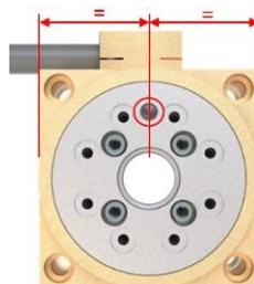
For the alignment of the rotor flange a single hole Ø4H7 is provided. With centric alignment of this hole on the side of the connector housing, the absolute zero point can be found.
